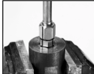
Fig. C15 — Fully tightened positioned with displaced mark
