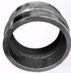
Example of Pipe Weld: 4" Carbon Steel, Sch 80
