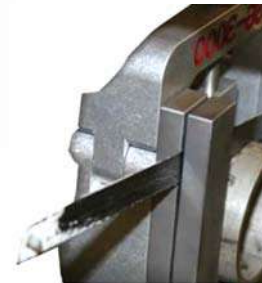
Pictured: example using Saw Guide to cut pipe/tube
