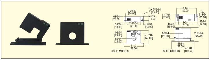
The Series CCT40/50 Current Transformers are a low cost alternative for measuring power and monitoring the operation of fans, pumps, or other equipment. For use on existing installations, split core models can be installed without disconnecting cables. Each model offers three jumper selectable ranges and a choice of three different outputs.
