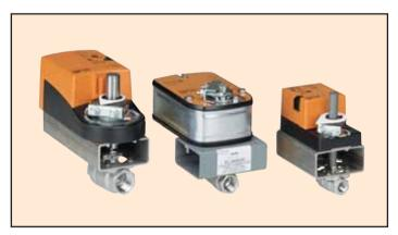
The Series BV2L is a low cost electric actuator combined with our durable two-piece stainless steel ball valve to make a compact, low cost, automated valve package. Electric actuators are available in either 24 VAC/DC or 120 VAC supply voltage. Spring return models return the valve to its failsafe position upon loss of power and are factory supplied to return to the closed position upon failure. The BV2L is an ideal valve package for HVAC applications and OEM's such as boiler manufacturers.
