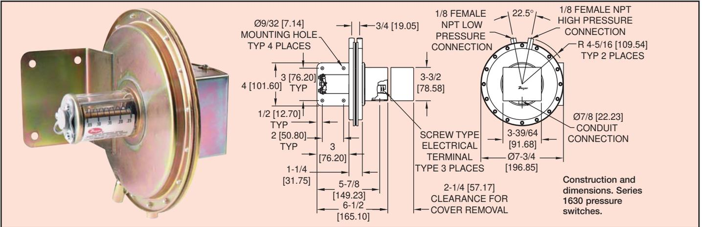
Our highest precision conventional large diaphragm pressure switch provides maximum dependability. In addition, it incorporates a visible set point indicator for maximum convenience. UL and CSA listed, FM approved for general service, these switches are suitable for most applications in air conditioning and industrial service. Electrical capability of 15 amps handles most small electrical loads.
